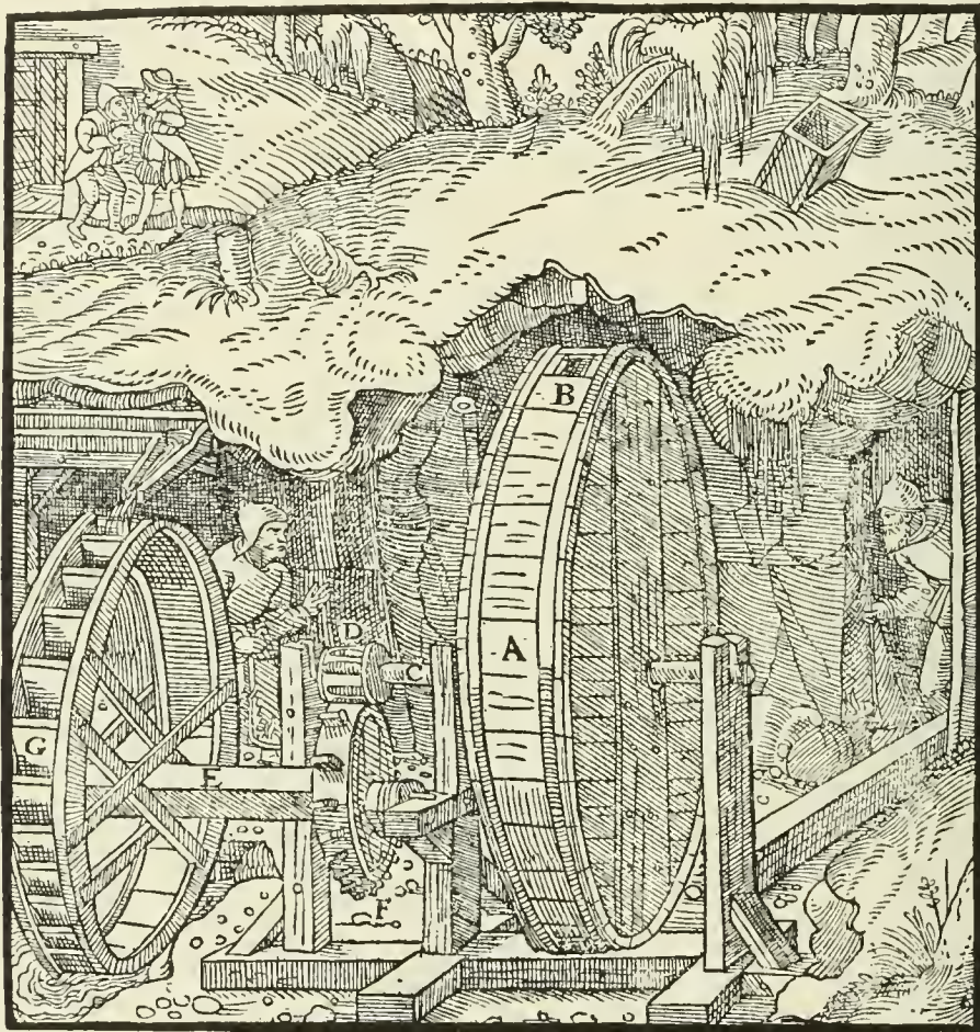
A—HOLLOW DRUM. B—ITS BLOW-HOLE. C—AXLE WITH FANS. D—DRUM WHICH IS MADE OF RUNDLES. E—LOWER AXLE. F—ITS TOOTHED WHEEL. G—WATER WHEEL.
